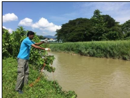
Figure 3.5: Collection of water sample using grab sampling method
