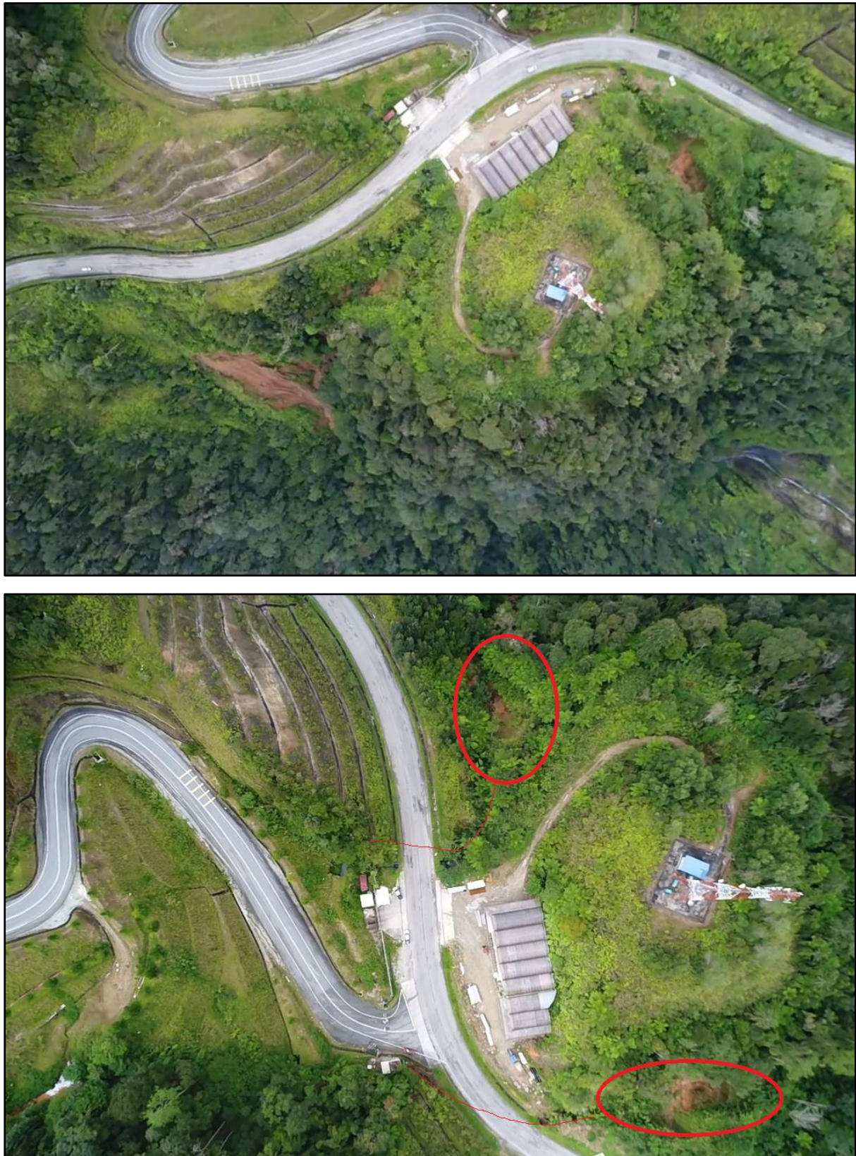
Figure 3.21: Two patches of slope erosion on either side of the Agroto Sdn Bhd store which shows the flow of the water from the drainage from the agro tourism site flowing contributing to slope erosion in the Kinta Catchment
