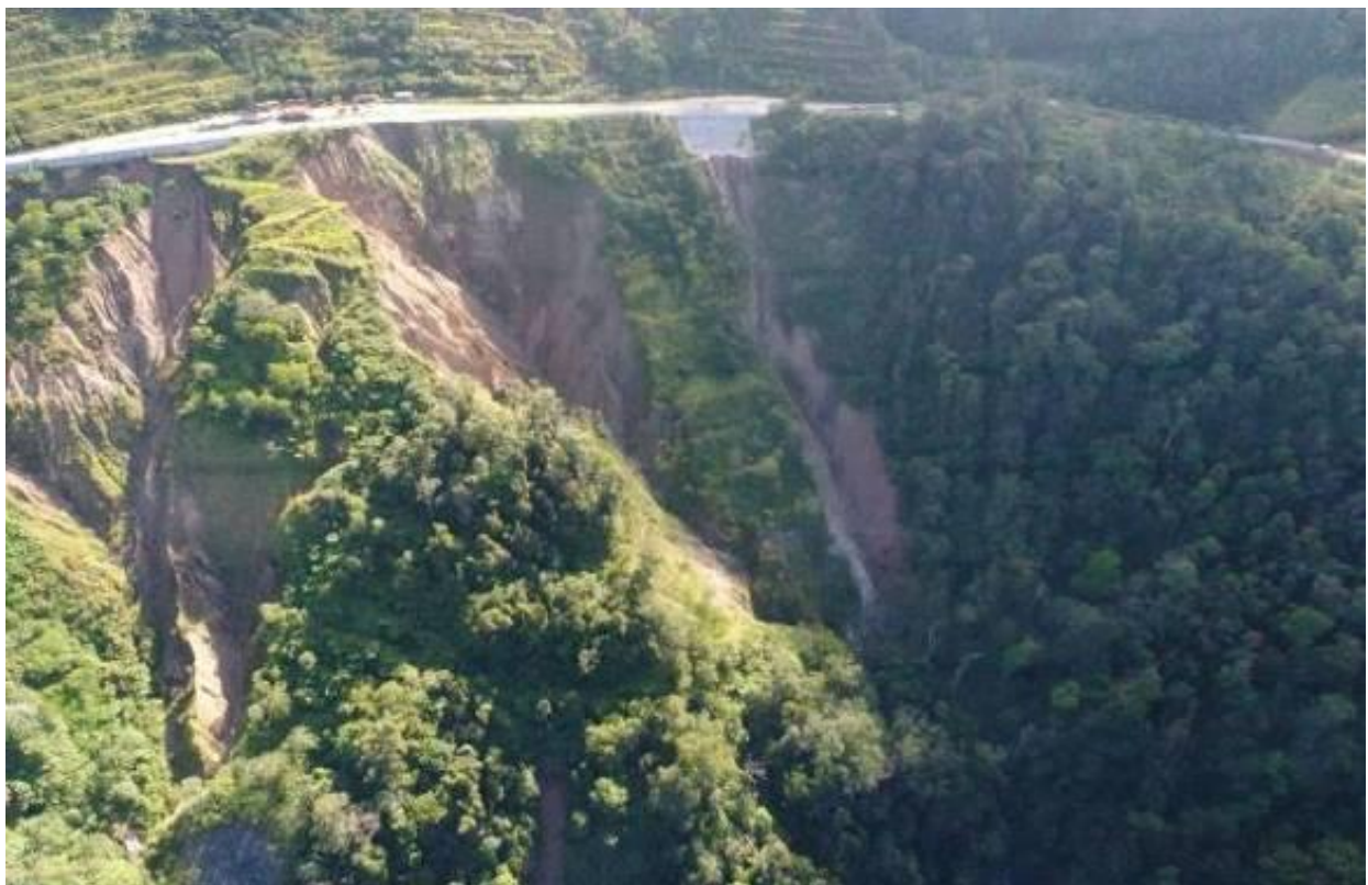
Figure 2.12 Landslide area at KM46, Simpang Pulai Highway, leading to sedimentation in Sg Penoh, hence to Sultan Azlan Shah Dam (captured on 24 February 2020)
