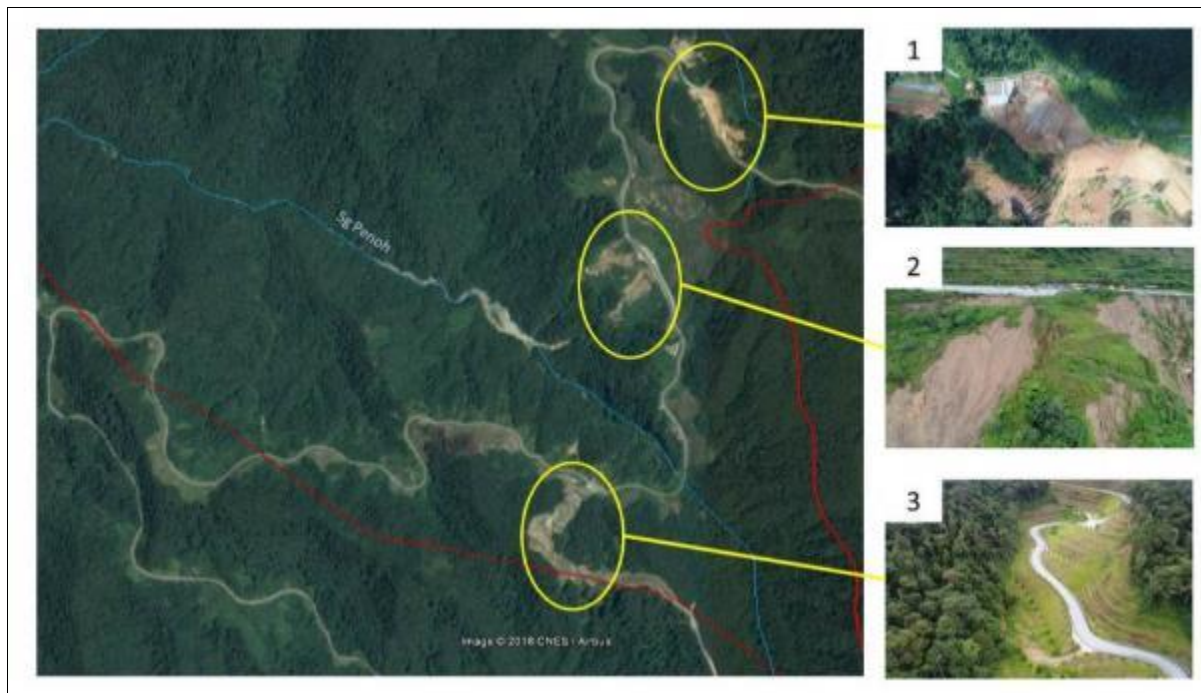
Figure 3.10 Satellite image and drone photo of the landslide and the erosion ending up into the Penoh River feeding into the Kinta River (Sultan Azlan Shah Dam) as in November 2018
