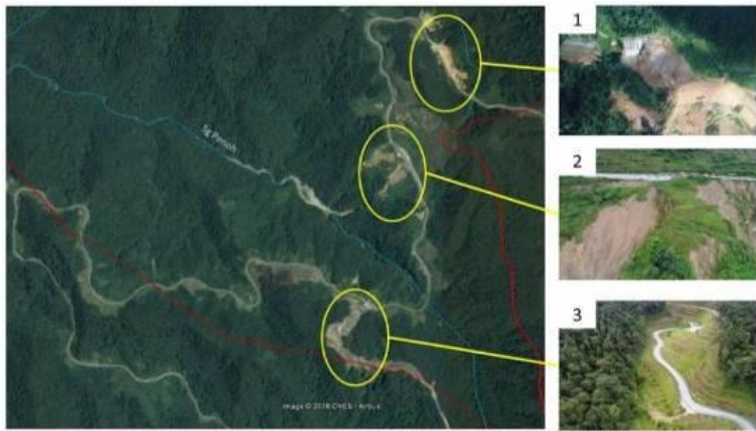
Figure 2.11: Satellite image and drone photo of the landslide and the erosion ending up into the Penoh River feeding into the Kinta River (Sultan Azlan Shah Dam)
