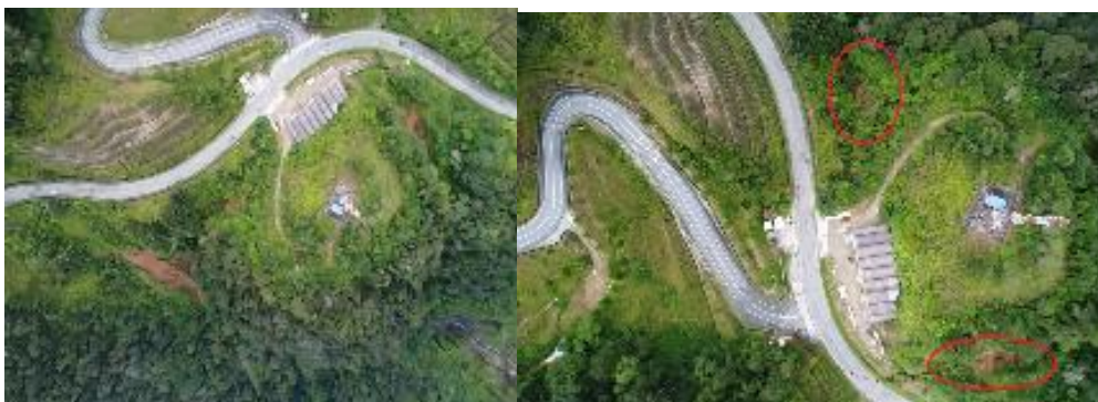
Figure 3.22 Two patches of slope erosion on either side of the Agroto Sdn Bhd store which shows the flow of the water from the drainage from the agro tourism site flowing contributing to slope erosion in the Kinta Catchment
